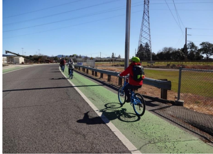
Figure SH.3. Green painted bike lanes on Valley View Street
