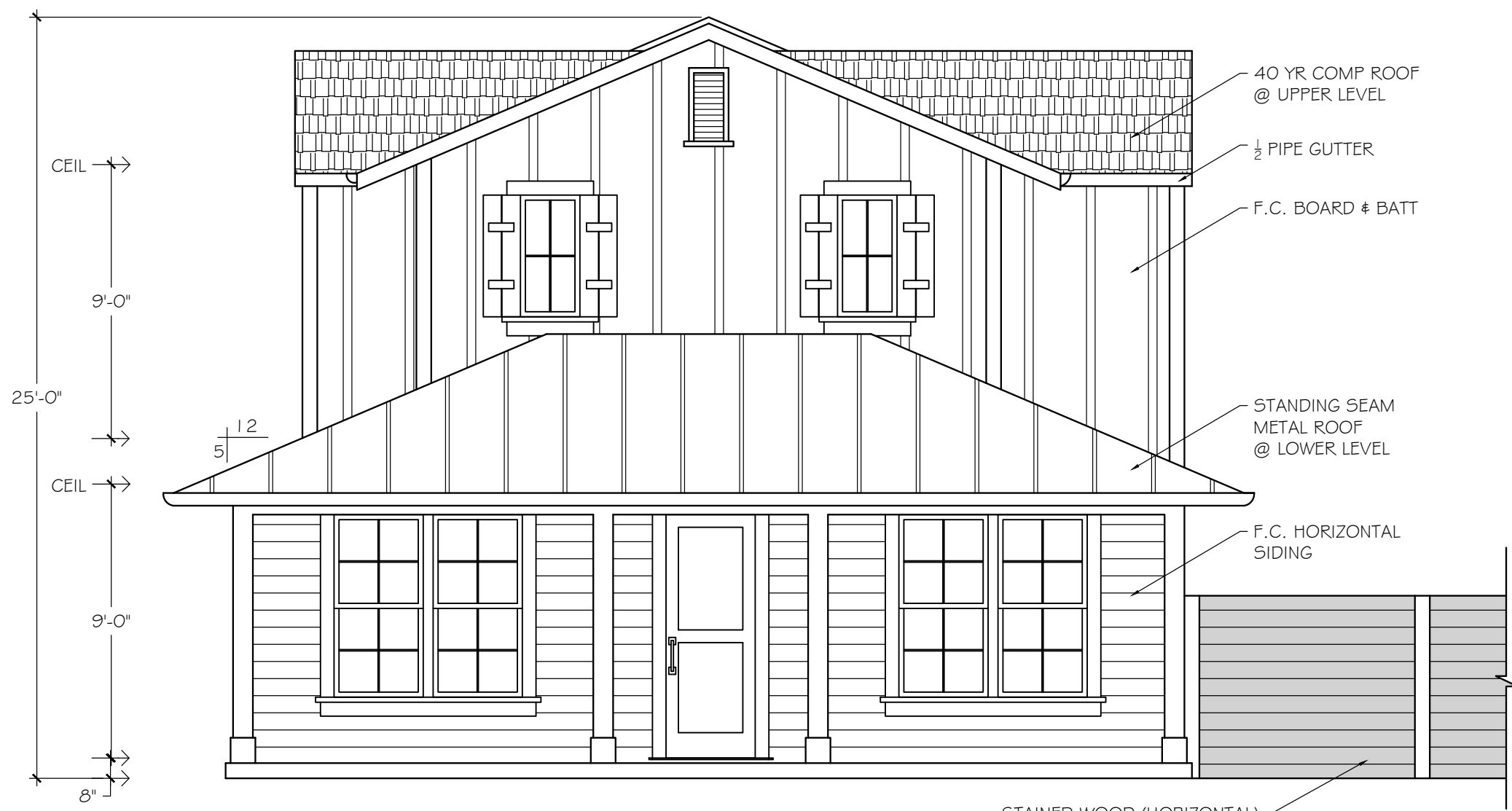
1 7 FRONT ELEVATION SCALE 1/4" = 1'-0"
