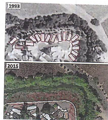
Figure 2 – The positive side of flood control. As part of the St. Helena project, a total of 17 mobile homes were permanently removed and the flood wall set back from the river.
