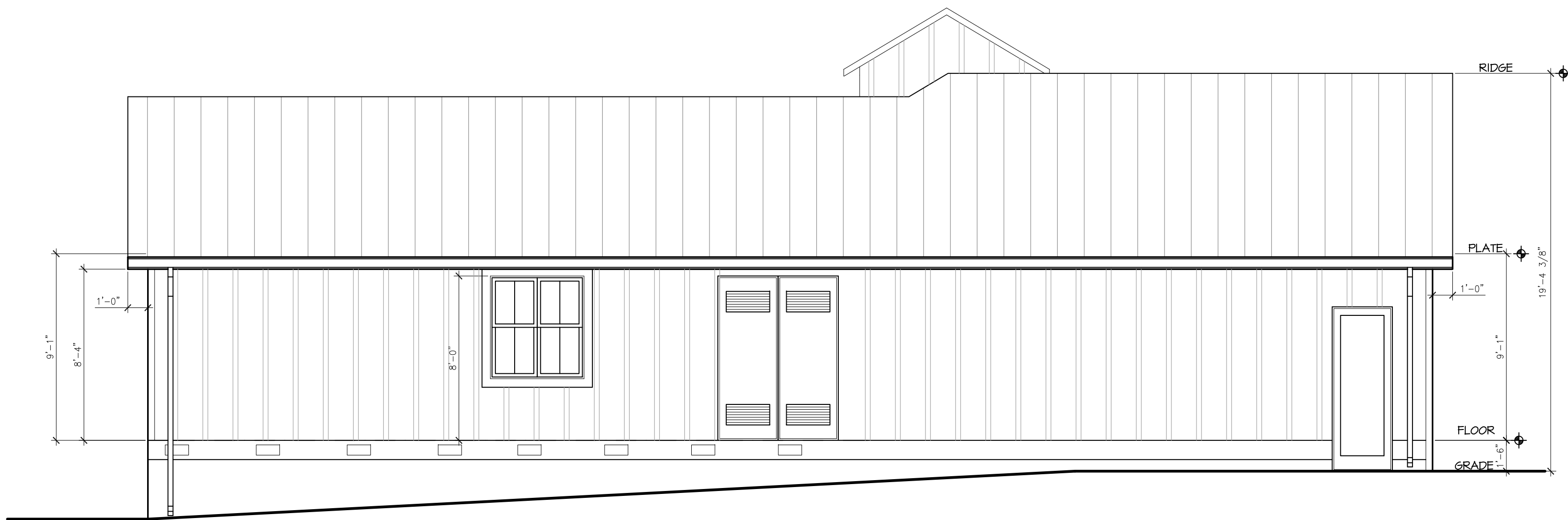
SIDE ELEVATION - NORTH SCALE: 1/4" = 1'-0"
