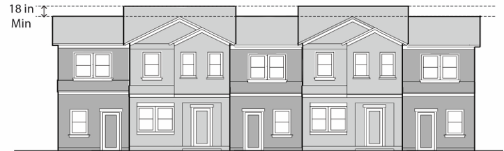
Figure 17.16.040.1j: Roofline, Attached Single Unit and Multi-Unit Development
