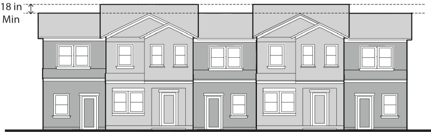
The roof line for each elevation shall be offset at least 18 inches for each one to three units exposed on that elevation.
