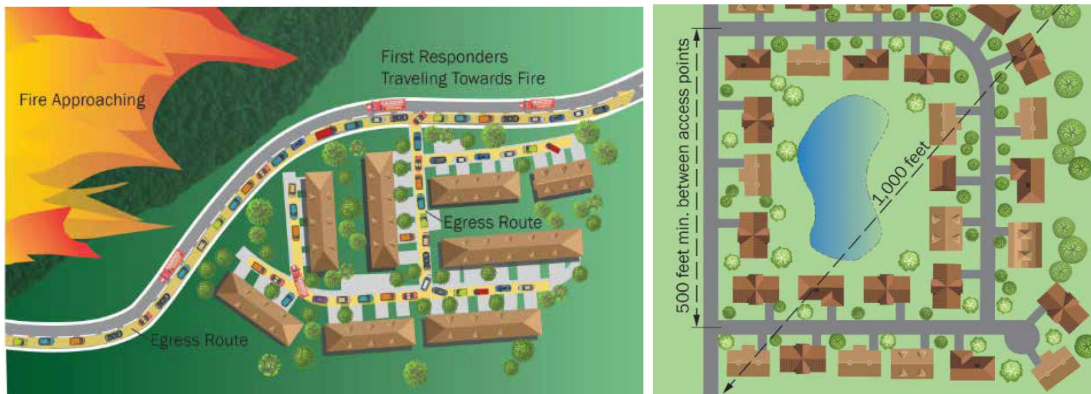
(Left) Schematic illustrating common life safety concerns and stresses affecting the general public, first responders, and the overall transportation network during major wildfire events. (Right) Diagram illustrating the concept of providing separate and independent egress routes from a neighborhood to improve evacuation safety during wildfire conditions.
