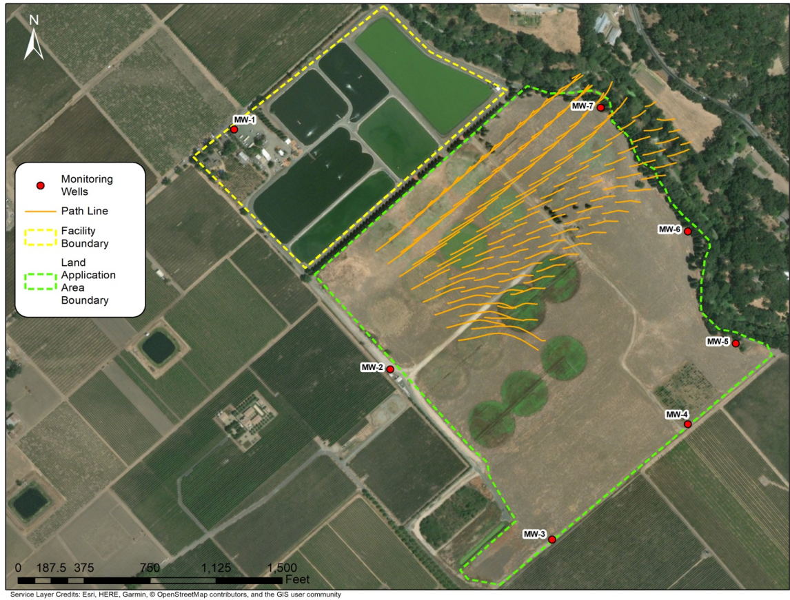
Figure 10. Recharged particle pathlines from irrigation on November 17, 2017, to April 19, 2018
