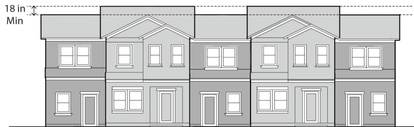
Figure 17.16.040.HJ: Roofline, Attached Single Unit and Multi-Unit Development
