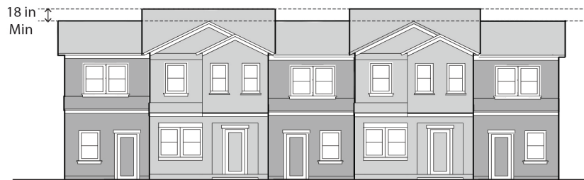
Figure 17.16.040.H: Roofline, Attached Single Unit and Multi-Unit Development
